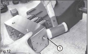
Remove the pump head (1, Fig. 12).
