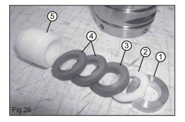
Fit each new component of the pressure packing set in the cylinder making sure of the correct order as shown in Fig 26:
