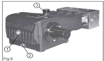
If necessary, top up from the oil plug 3, Fig. 8.
