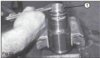
In order to replace the fackings, firmly hold the cylinder and loosen the packing support nut (1, Fig. 22).
