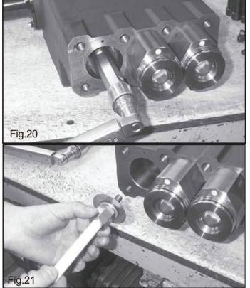
Once the cylinders are removed, loosen the plungers and check them for wear (Fig. 20 and 21). Replace if necessary.
