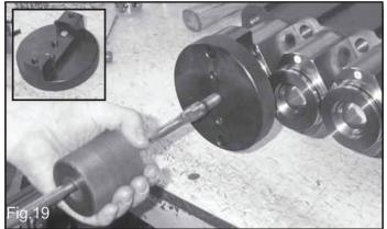
Once the head is removed the cylinders are free to be taken out of the crankcase. Tapping the cylinders all around with a plastic hammer helps loosen them from possible scaling or deposit accumulated during use. In order to facilitate the extraction of the cylinder the tool p/n F200000180, or equivalent, is recommended (Fig. 19).
