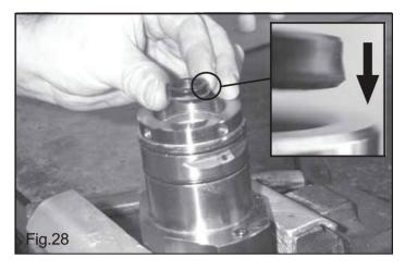
Fit the packing support nut back in place and tighten. The new rear seal should be mounted with the larger diameter side in first, as shown in Fig. 28.
