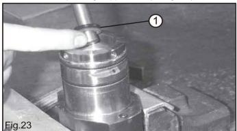
Using a pin of adequate dimensions take out the rear seal (1, Fig. 23).
