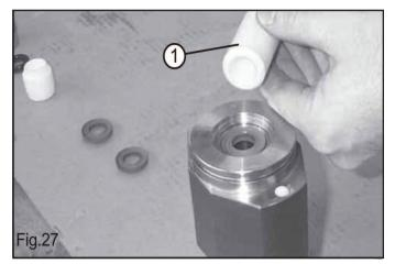
Each pressure packing set component should fit tight in the cylinders. A pin of adequate dimension (1, Fig. 27) helps in guiding each component straight and aligned all the way down the cylinder.
