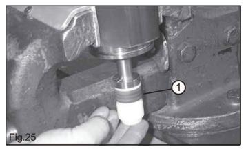
Turn the cylinder upside down, hold it vertically, insert a pin of adequate dimensions (1, Fig. 24) and smartly tap until the complete pressure packing set is out (1, Fig. 25). The pressure packing set (1, Fig. 25) hould be replaced at every disassembling.
