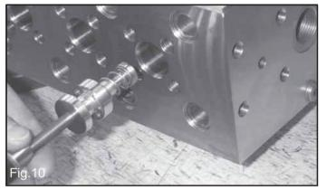
Once removed take out the delivery valve guide with the spring and valve poppet. AN M8 threaded bolt to be used as a simple extractor would help the operation (see Fig. 10).
