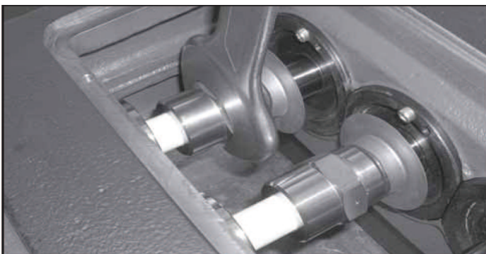
Once head and collector are removed the cylinders (1, Fig.21) are free to be taken out of the pump body. Tapping the cylinders all around with a plastic hammer helps to loosen them from possible scaling or deposit accumulated during operation.
