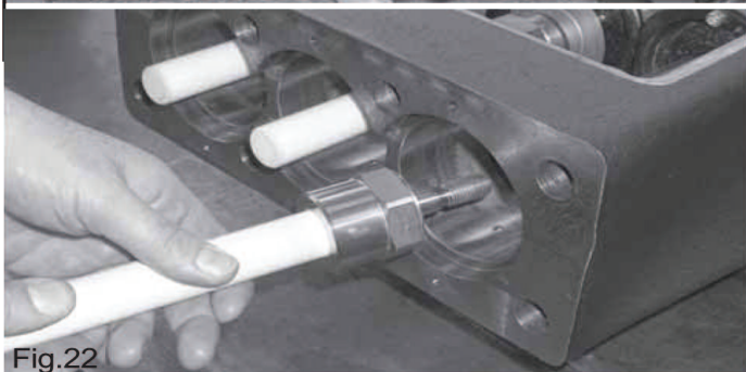
Once the cylinders are removed, loosen the plungers and check them for wear (Fig 22). Replace if necessary.
