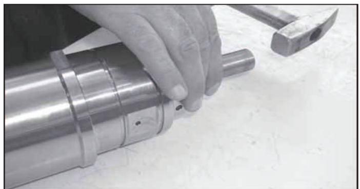
Remove the rear support 1, the rear seal 2 and the o-ring (3, Fig. 24).
