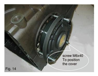
E) Fit the back cover putting the dipstick hole upward.
