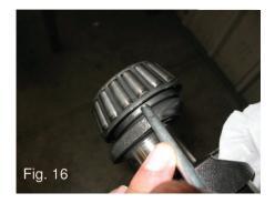
The new roller bearings can be mounted at room temperature with a press; it is necessary to hold them on the side surface of the ring nuts with suitable rings. The driving operation can be facilitated by heating the parts at a temperature between 250-300<sup>O</sup>F, making sure that the ring nuts are correctly fitted in their seats. Note: Take care not to invert the components of the 2 bearings (outer ring nut of bearing 1 instead of the one of bearing 2...).
