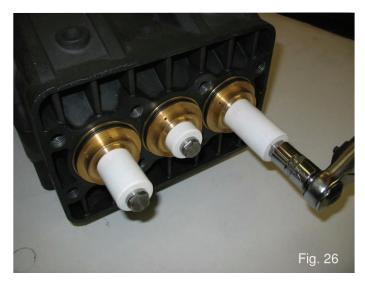
A) Loosen and remove the plunger screw (1, Fig. 26).
