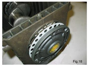
F) If the torque is correct, connect the rods to the crankshaft, otherwise, calculate the shims again as per point "C".
