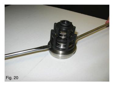
Check the components for weat and replace if necessary. **Replace all o-rings of the valve units and plugs, at each inspection.**
