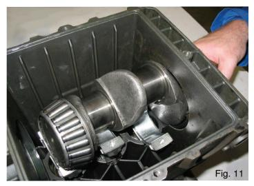
C) Before reassembling the side covers, check the seal lips for wear. If they need replacing, fit the new ring following the indications in Fig. 12.
