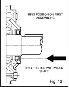
Note: Should the shaft show diameter wear in the seal position, it is possible to avoid grinding it by fitting the seal further as indicated in Fig. 12. Before installing the cover, (sight glass side) check the shim rings have been placed. To help the covers fit on the crankcase, you can use 3 screws M6 x 40, and then finish screwing them with the original bolts (M16 x 18).
