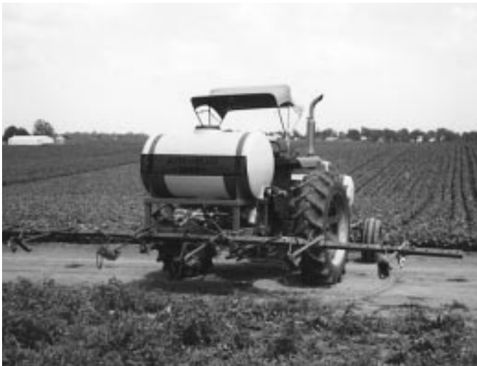
Seven spray arms operate simultaneously injecting fertilizer through the "0" nozzles at 2200 PSI.
