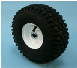
1225 Tire, 10.5" dia full pneumatic, 3/4" bore, knobby tread.
