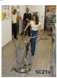
VacuBerm reclaims to 15 gpm with a shop vacuum.
