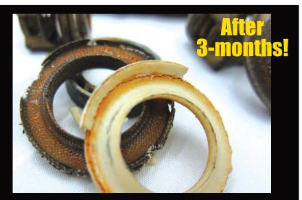
The customer bought two of these pumps and when they stopped working after 3-months I just had to see why. You don't even have to look 'close' to see that the packings are melted and pistons are *burnt to a crisp.*'
