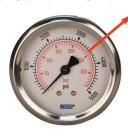
**SPIKE** pressure should never be more than 15-20% of operating pressure. This means that if your operating pressure is 3,000 PSI then your spike pressure should not exceed a maximum of 15-20% or, in this
