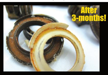
The customer bought two of these pumps and when they stopped working after 3-months I just had to see why. You don't even have to look 'close' to see that the packings are melted and pistons are 'burnt to a crisp.'
