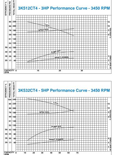
All calculations based upon water @ Spec. Gravity of 1.00
