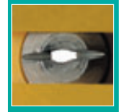
STAINLESS NOZZLE AFTER 50 HOURS
