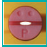
CERAMIC NOZZLE AFTER 50 HOURS
