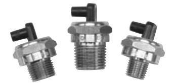
Protects the pump from damaging heat build-up while it is in bypass mode. The thermal relief valve, sensing a rise in temperature, opens and discharges a small amount of heated fluid. This allows cooler water to enter the system and cool the pump. When the gun is discharged the cooler water will cause the valve to close immediately.
